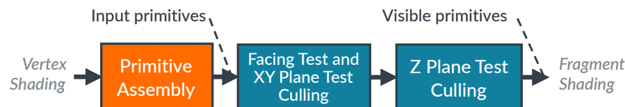
Figure 4-1: Midgard GPU culling pipeline
